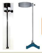
Tared piston and tripod mount of the device for equivalent of sand
